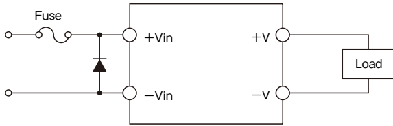
Figure1-5 Protection for Reversed Connection of Input
